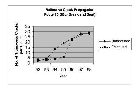
Figure 4. Reflective Cracking Over Time for Site 4, Reinforced Concrete Slabs
