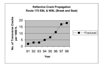
Figure 5. Reflective Cracking Over Time for Site 5, Reinforced Concrete Slabs
