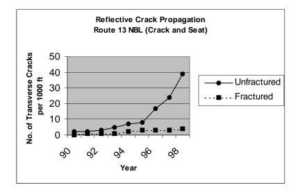
Figure 1. Reflective Cracking Over Time for Site 1, Unreinforced Concrete Slabs
