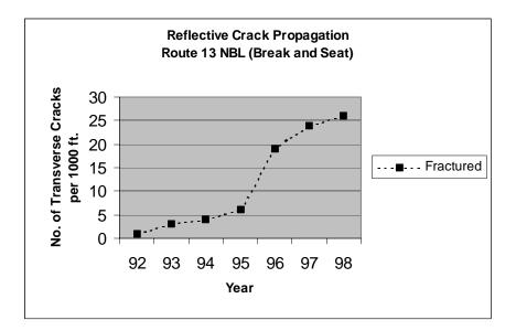
Figure 3. Reflective Cracking Over Time for Site 3, Reinforced Concrete Slabs
