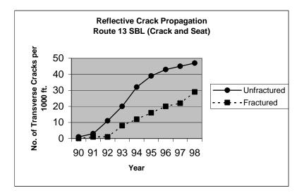
Figure 2. Reflective Cracking Over Time for Site 2, Unreinforced Concrete Slabs
