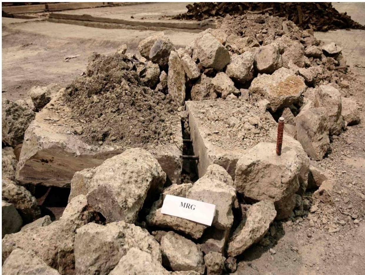
**Figure 4.4, Excavated Rubblized PCC in MRG Section at NAPTF [Garg ppt, 2006]**
