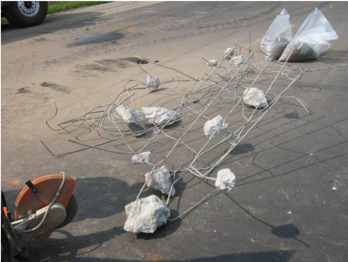
**Figure 5.1, Substantial Debonding of the Steel Rebar**
