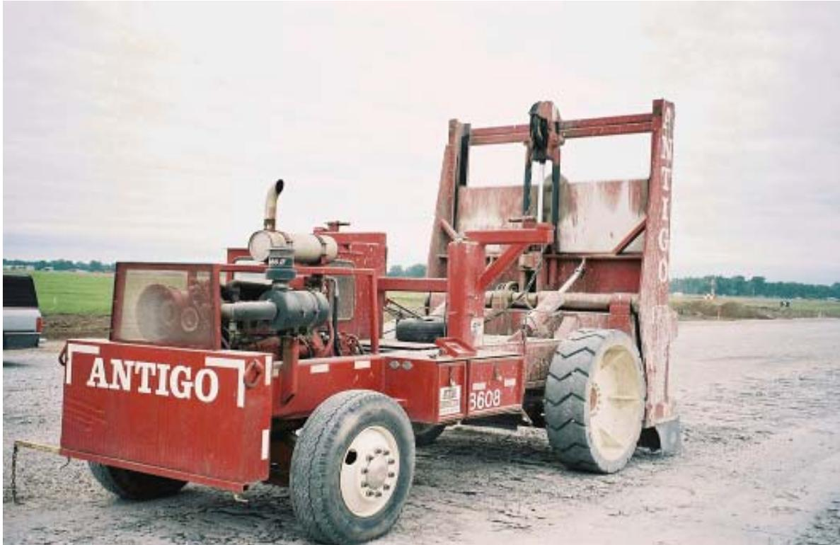
**Figure 3.12, Guillotine Hammer Used with Traditional Crack and Seat Method**
