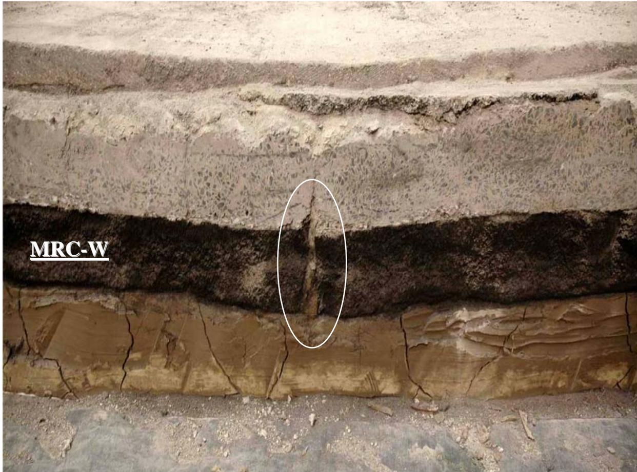
**Figure 2.6, Close-up in MRC Trench Showing Subgrade Shear Failure (Garg, 2006)**
