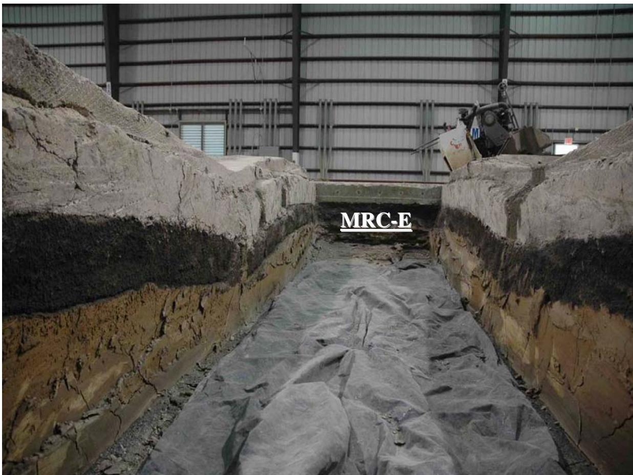
**Figure 2.5, Trench in MRC Showing Subgrade Shear Failure [Garg, 2006]**
