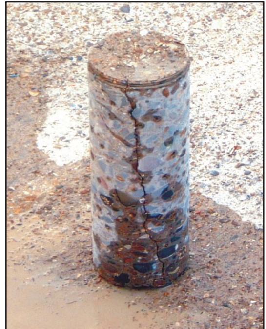
Fine vertical crack, induced with a single strike of the 8600 guillotine blade
