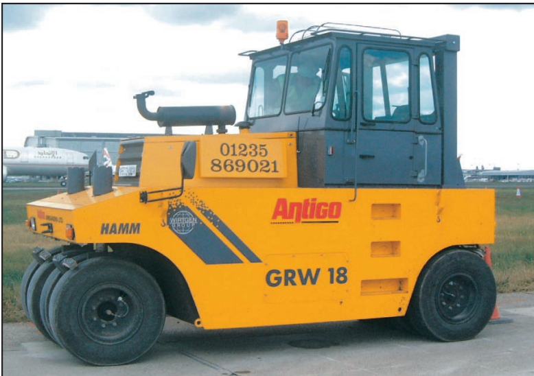
Typical pneumatic rubber tyre roller utilized for the seating operation [min weight 20 tons]
