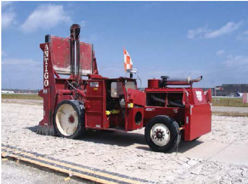
8600 Badger Breaker® breaking concrete
