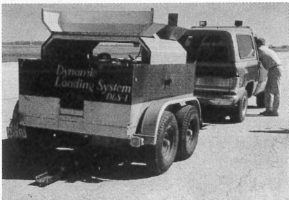
Nondestructive testing equipment being operated by Roy D. McQueen & Associates crew.
