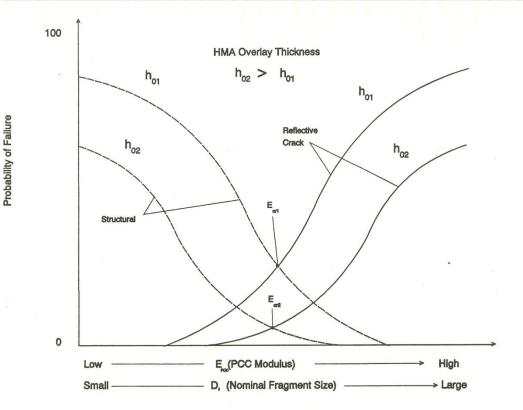
FIGURE 62 INFLUENCE OF PCC FRACTURED MODULUS AND HMA OVERLAY THICKNESS UPON STRUCTURAL AND REFLECTIVE CRACK FAILURE
