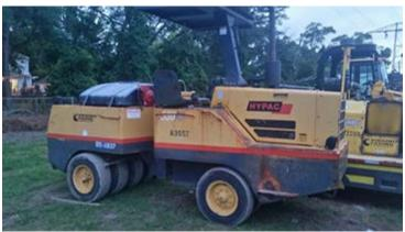
Figure 8. Rubber Tire Roller
