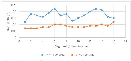
Figure A6. Rut Data for SR 406 (Westbound). PMS = Pavement Management System.
