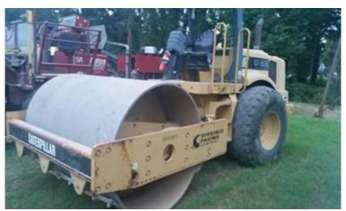
Figure 9. Steel Drum Roller
