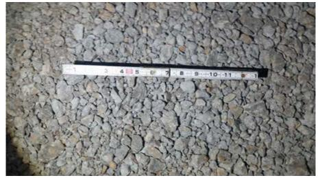
Figure 10. Aggregate Particle Size After Z-Roller Compaction
