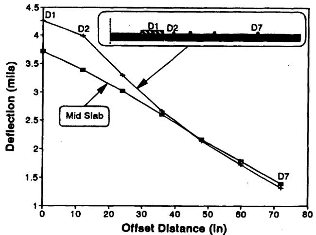
**FIGURE 6** Effect of cracks/joints on surface deflection (Configuration 1).
