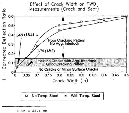
FIGURE 9 Effect of crack width on FWD measurements.
