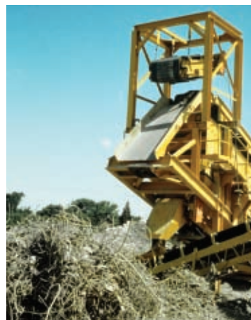
Figure 13. Removal of reinforcing steel on the job site or after crushing.
