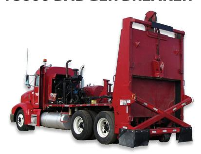
The **T8600 Badger Breaker**® is a truck-mounted, guillotine-style concrete pavement breaker which carries a 8-foot (2.4m) wide, 12,000 pound (5,500kg) hammer. The lift height of the hammer is electrically adjustable from 0 to 9 feet (2.7m).
