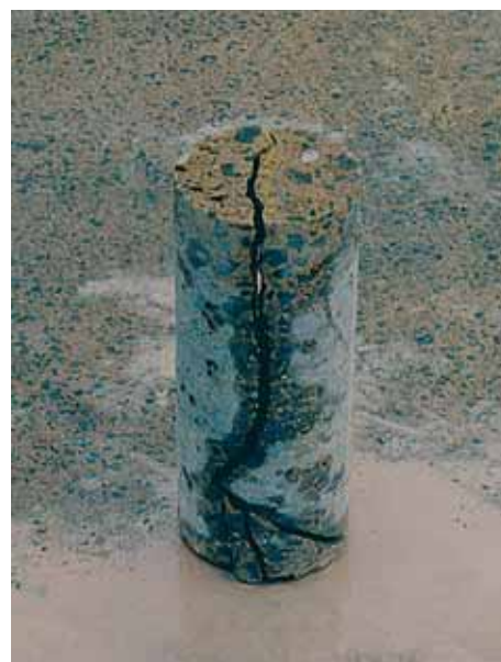
Plate 6.9 Over-cracked, vertically branching crack
